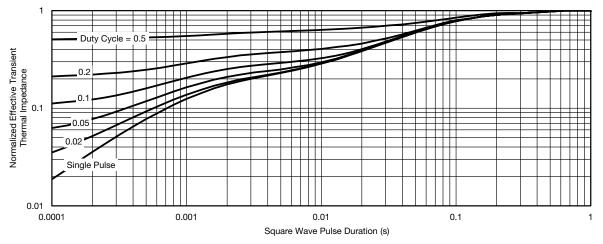
Normalized Thermal Transient Impedance, Junction-to-Case
