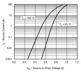
Source-Drain Diode Forward Voltage
