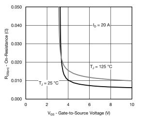
On-Resistance vs. Gate-to-Source Voltage
