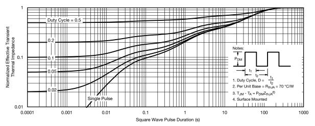
Normalized Thermal Transient Impedance, Junction-to-Ambient
